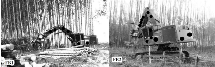
FIG. 1 Crawler Feller-buncher without leveling device – FB1; Crawler Feller-buncher with leveling device – FB2
