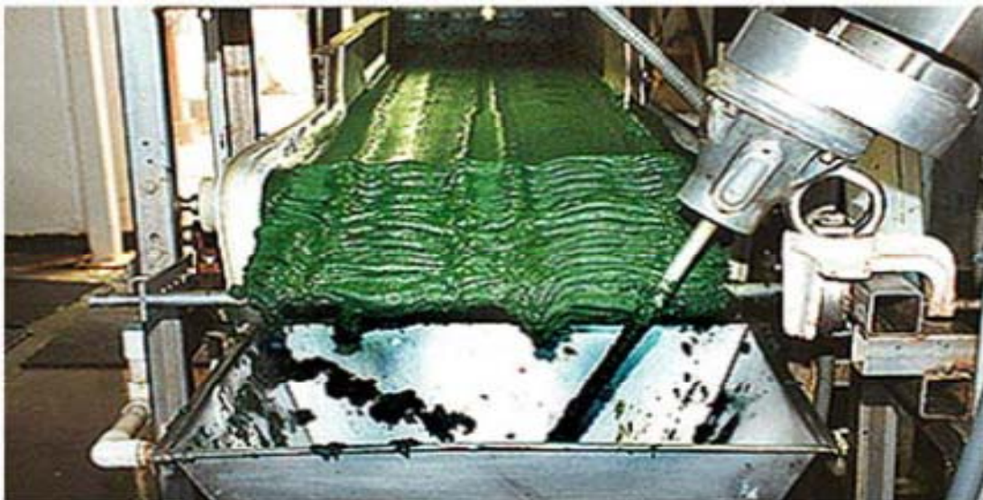
Figure 2: Microalgal biomass recovered from the culture broth by filtration
