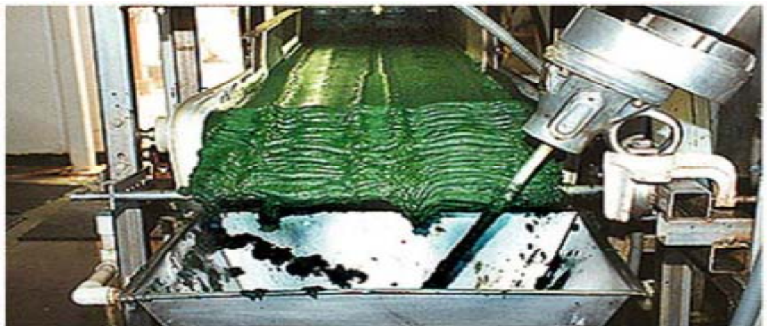
Figure 3: Microalgal biomass recovered from the culture broth by filtration (Source: Oilgae, 2014)
