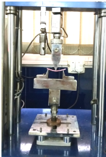
Fig. 2 - Testing the specimen on Universal Testing Machine
