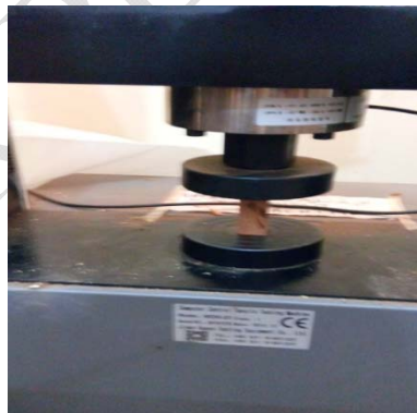
Figure 1: Maximum Compressive Strength (MCS) parallel to grain test on a Universal Testing Machine
