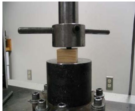
Figure 2: Determination of Hardness using Janka tester
