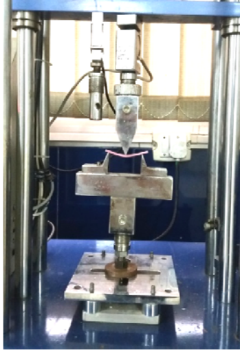
Fig. 2 - Testing the specimen on Universal Testing Machine
