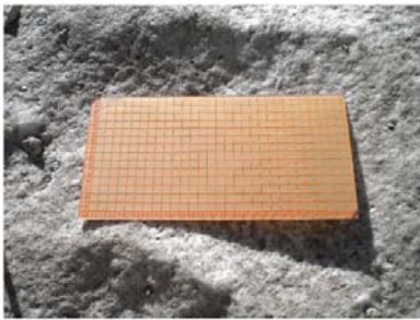
Fig. 2: The surface profiler used to estimate size of the debris during the field study over the Chhota Shigri glacier.
