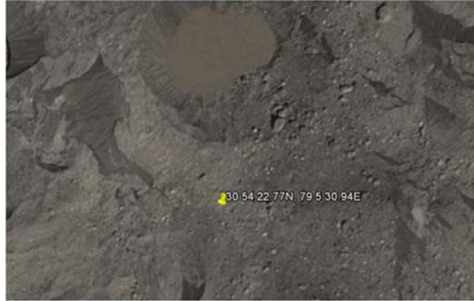
Fig. 6: Google earth image of 26th September 2014. The average debris size at the highlighted location is estimated as 480 mm. From the classification output the size is detected as 521 mm.
