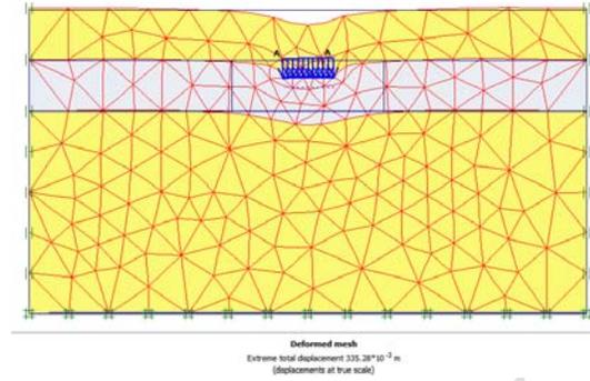
**Fig. (3) Deformed mesh for compacted sand layer**
