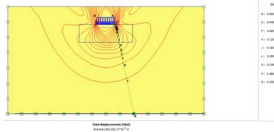
**Fig. (4) Total Displacement contours for loose sand**
