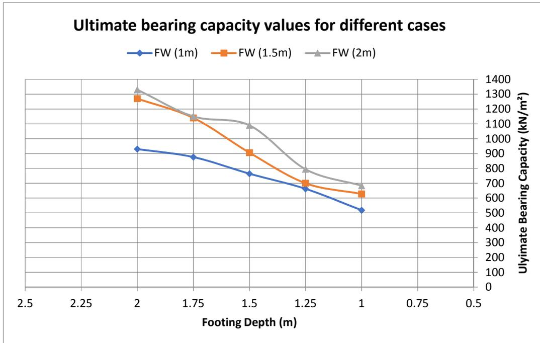
**Fig. (9) Ultimate bearing capacity vs Footing Depth for different cases (optional)**
