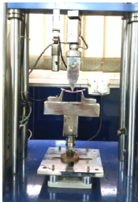
138 Fig. 2 - Testing the specimen on Universal Testing Machine
