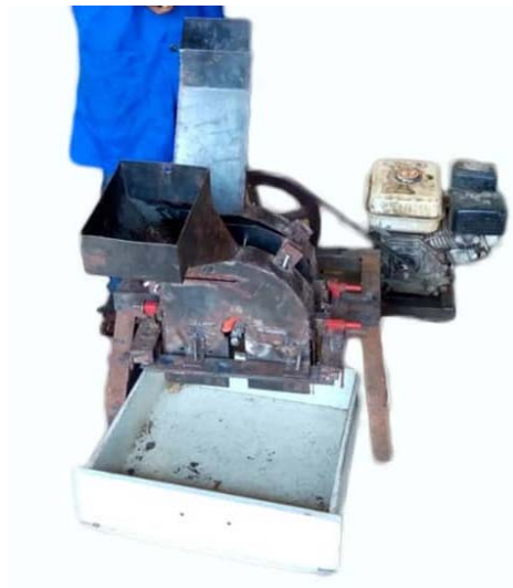
Figure 1: The pictorial view of the portable ginger slicing machine
