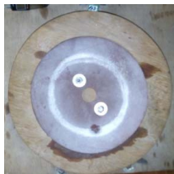
Fig10: Disk with the Emery Paper
