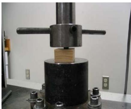
Figure 2: Determination of Hardness using Janka tester
