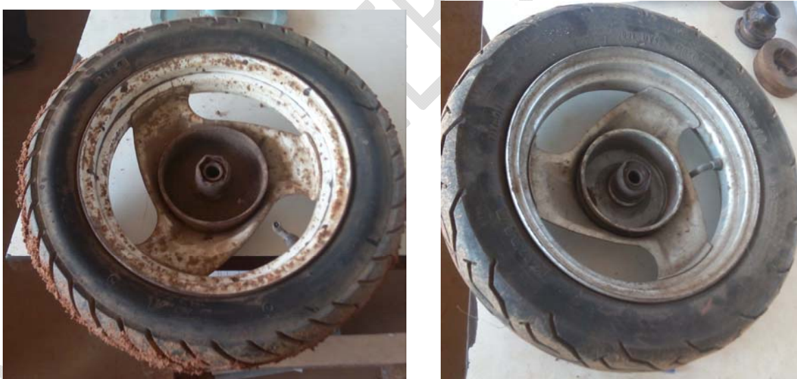
162 Figure 3. Test wheel one (1) and test wheel two (2) showing different thread design
