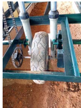
Figure 2: Drive unit view showing the towing cable, coupling of trolley to the carriage and wheel tester
