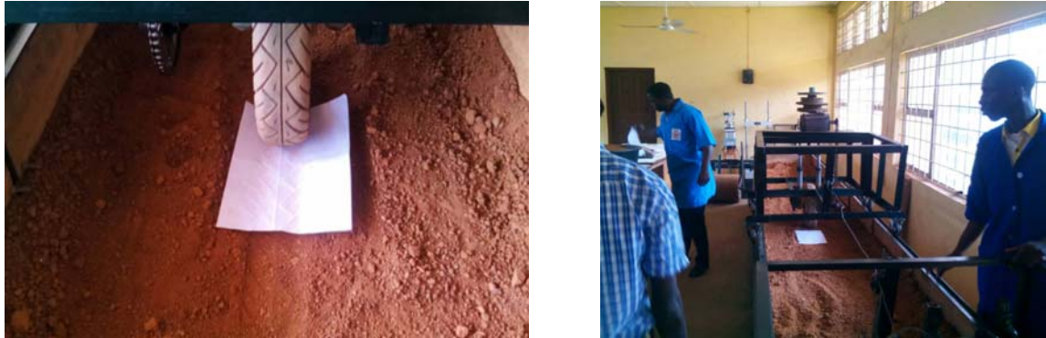
168 169 Figure 4. Testing of the Test Rig to get the effect of load on the Motion resistance and 170 contact area with soil.
