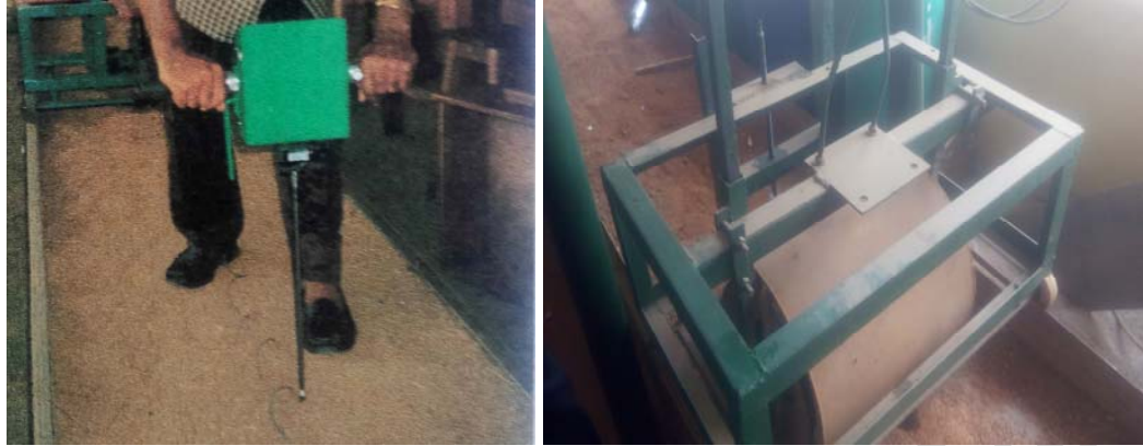
Figure 1. Soil penetrometer and Compaction roller
