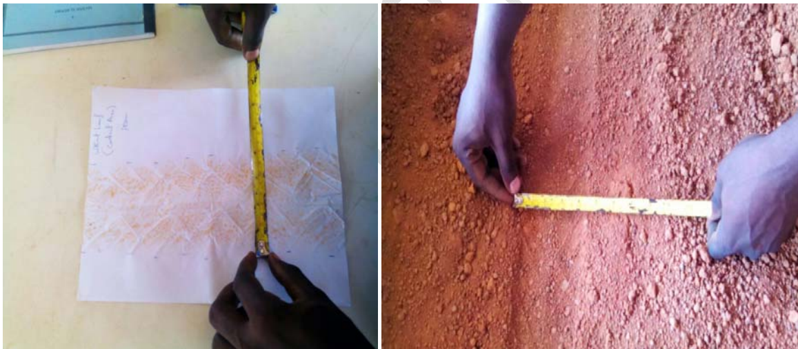
171 172 Figure 5. Measuring the Effect of load and inflation pressure on the contact area with soil.
