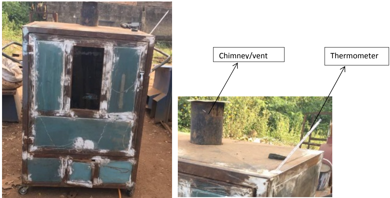
Fig. 3: Fabricated Gas Oven
