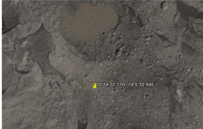
103 104 Fig. 6: Google earth image of 26th September 2014. The average debris size at the 105 highlighted location is estimated as 480 mm. From the classification output the size is 106 detected as 521 mm. 107
