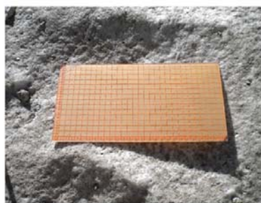
63 Fig. 2: The surface profiler used to estimate size of the debris during the field study over 64 the Chhota Shigri glacier.
