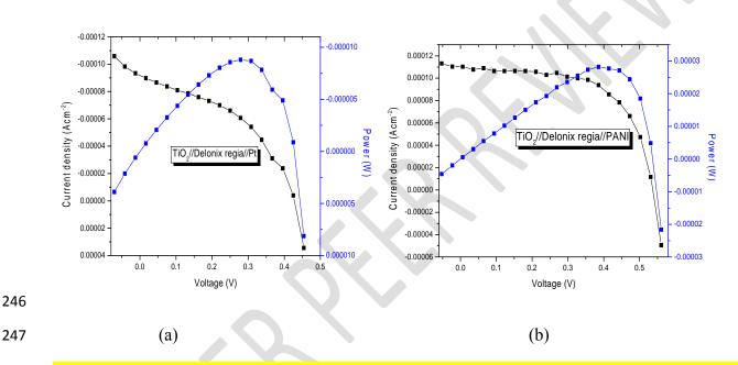
Fig. 4. Current density ( $J_{SC}$ ) and Power (W) versus Voltage (V) for (a) TiO<sub>2</sub>-DSC//*Delonix regia dye*//Platinum electrode and (b) TiO<sub>2</sub>-DSC//*Delonix regia dye*//PANI electrode.
