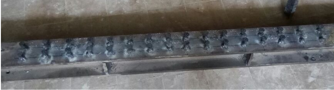
a- Shear connectors with 10 mm diameters welded above the compression flange
