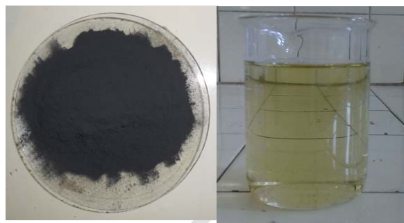
Figure 2 : Electrode material powder and leaching filtrate
