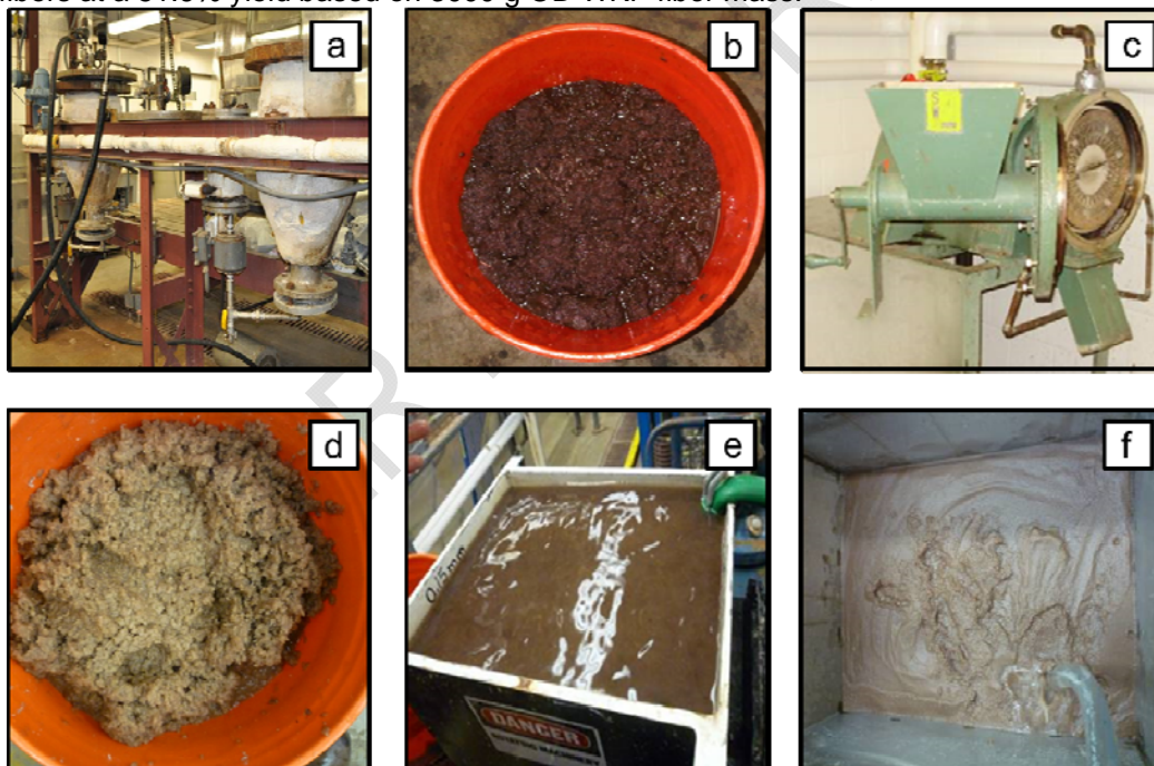
Fig. 4. WKP processing a) 3 cuft digester, b) WKP pulping, c) Sprout-Bauer Refiner, d) refined WKP, e) WKP screening, e) WKP fibers [35]
