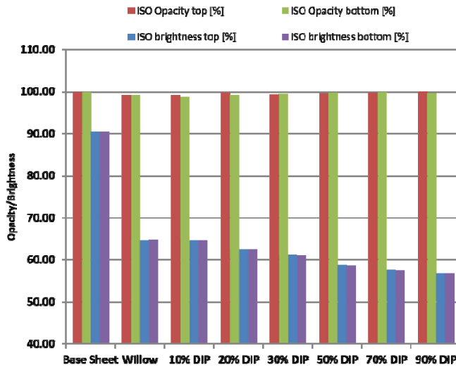
Fig. 15: 12” Pilot Paper Machine Paper Properties: Brightness and Opacity
