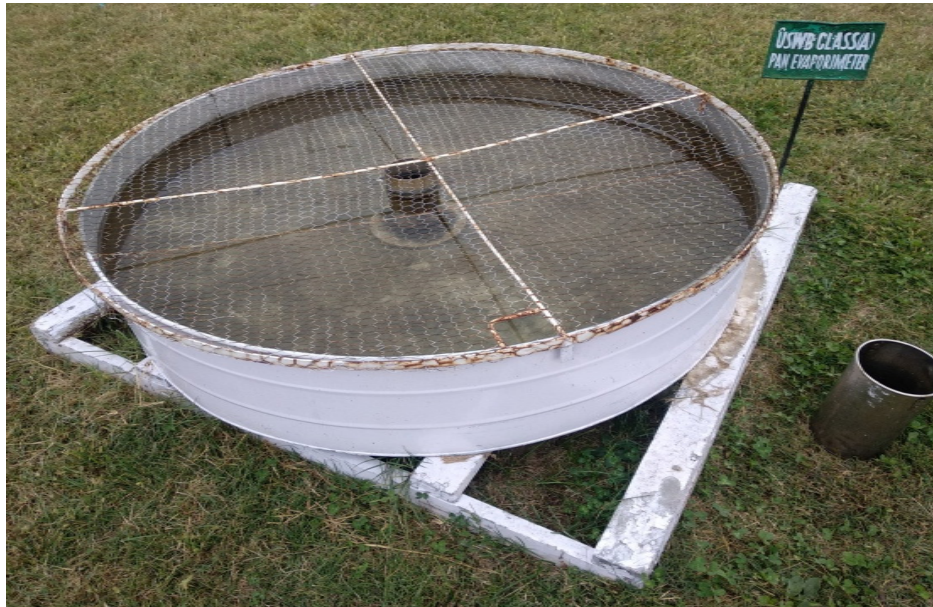
Fig 3: USWB CLASS(A) Pan Evaporimeter installed at Agromet station of SKUAST-Kashmir
