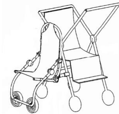
197 Figure 13: Baby stroller invented by Schutzendorf and Griffith [25].
