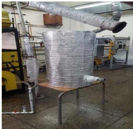
Figure 14: Experimental set up - Waste Heat Recovery from Diesel Engine
