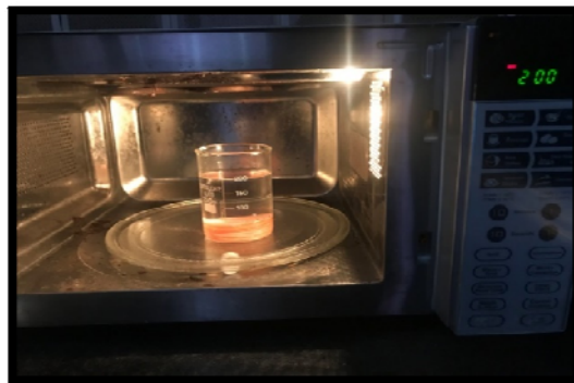
Fig. 4. Sample placed in microwave for 2 min at 430 W
