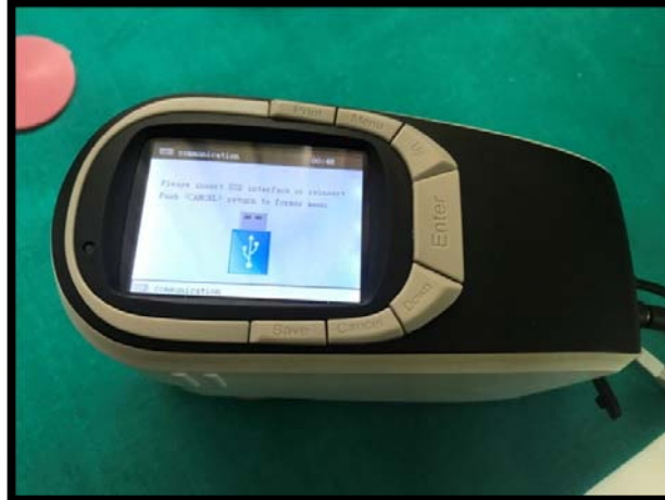
Fig. 5. Spectrophotometer Color Guide 45/0 used for Sample testing
