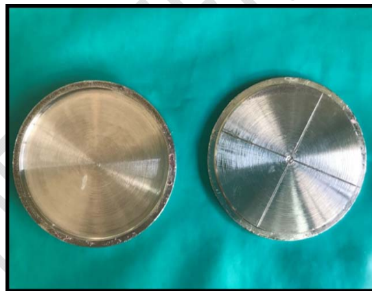
Fig. 1. Stainless Steel Die (ADA Specification no. 19)
