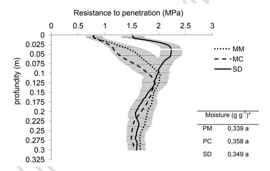
Figure 1. Soil penetration resistance (MPa) of each soil management, evaluated at 97 (DAS) in the 0-0,3 m layer in wheat irrigated in Tangará da Serra, MT. The bars indicate the standard error values of the mean and the overlap of these denotes the absence of differences between the means of the treatments. \* Means followed by the same letter do not differ from each other, by the Tukey test (p <0.05).
