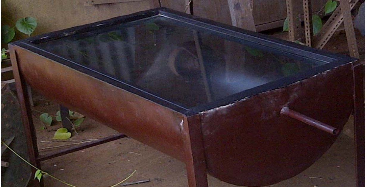
Figure ii: Thermal Storage Chamber
