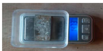
Fig. 4. Ultrasensitive weighing balance used for weighing the cast steel coupon.
