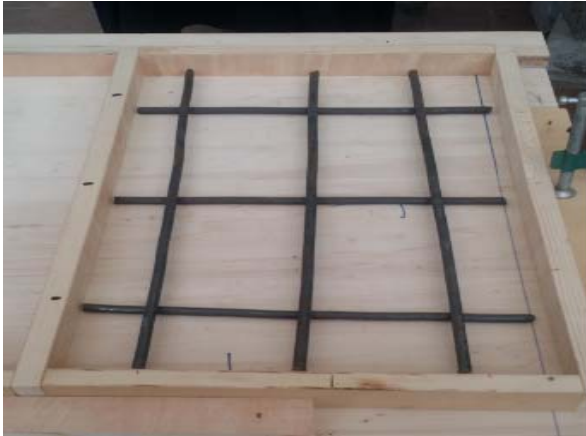
Fig (4) Rectangular footing model with steel reinforcement
