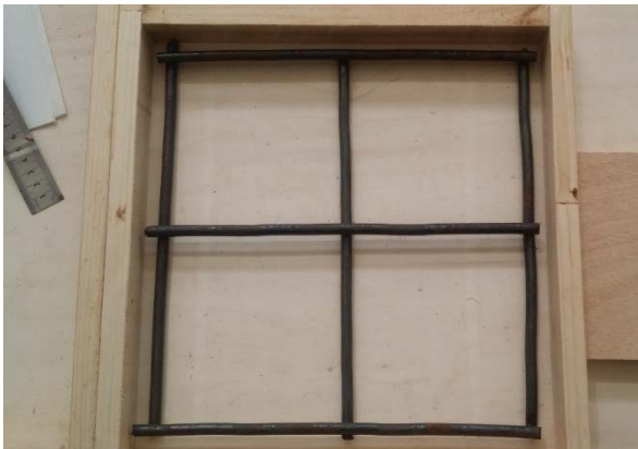
Fig (5) Square footing model with steel reinforcement
