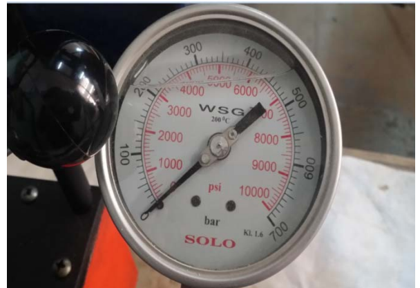
Fig (7) Dial gauge of the hydraulic jack of loading
