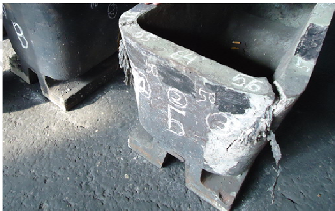
Figure 1. A broken down mold with leaked alloy traces.
