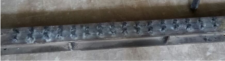
151 a- Shear connectors with 10 mm diameters welded above the compression flange
