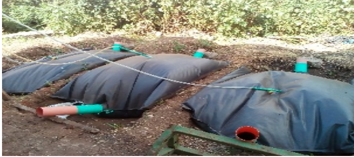
Fig 1: Miniature Biogas digesters set up at JKUAT
