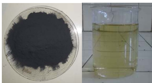
Figure 2: Electrode material powder and leaching filtrate
