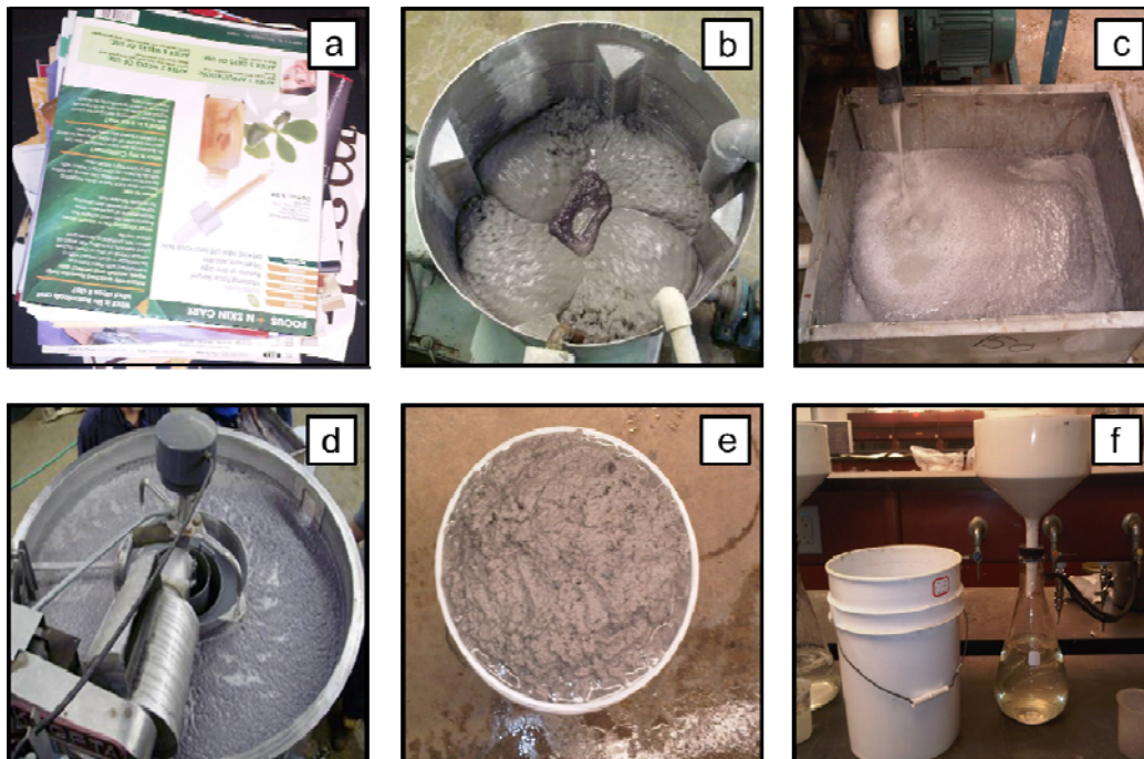
Fig. 3. DIP processing a) ONP & OMG, b) hydro pulping, c) ink removal, d) flotation, e) pulp storage f) dewatering [32]
