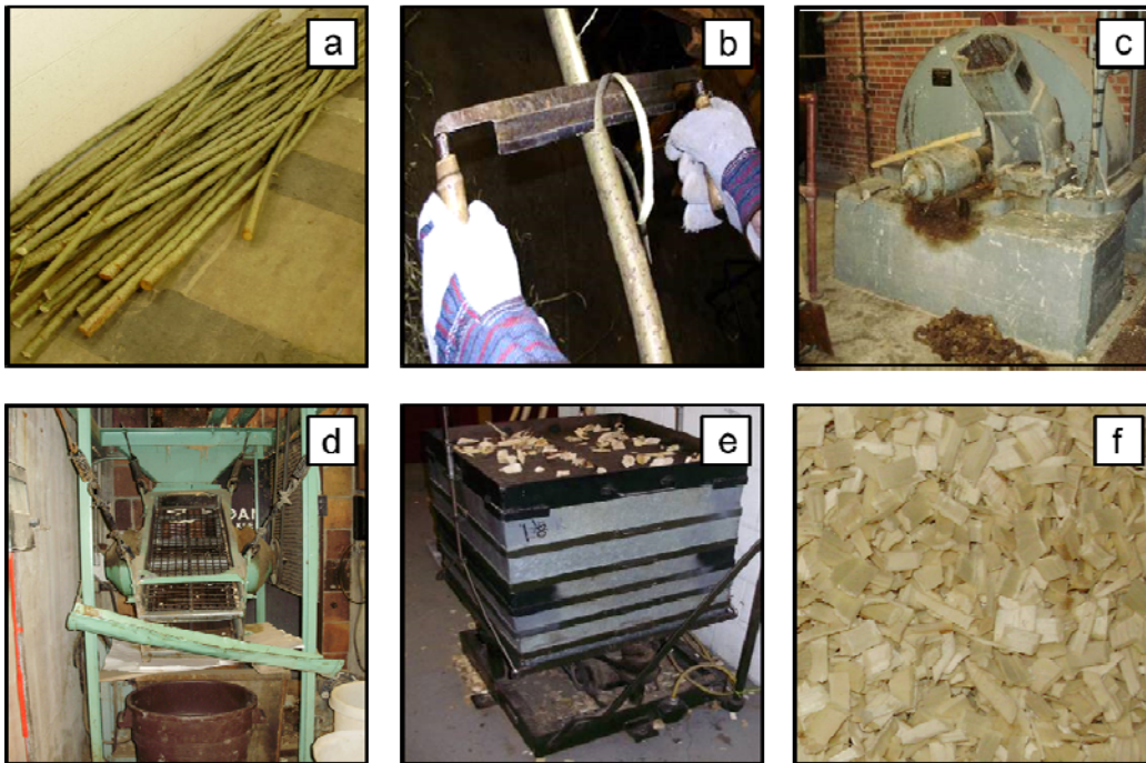
132 133 Fig. 1. Willow processing a) willow stems, b) debarking, c) chipping, d) pre-screen, e) 134 final screening f) willow chips [31] 135
