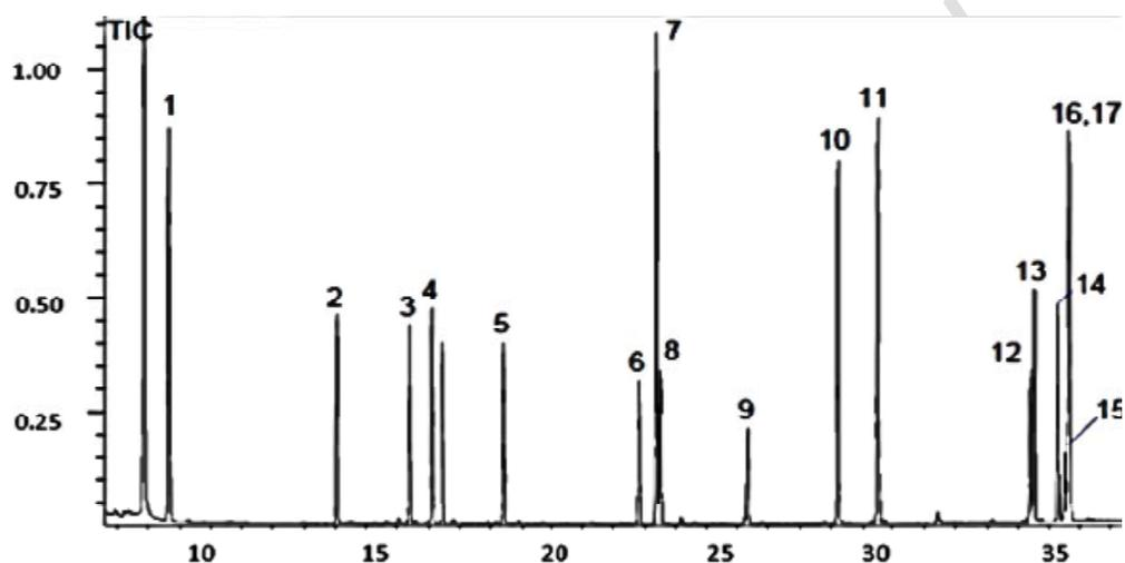
Fig. (3) Retentions times (Rt) for SRM mode GC-MSMSTQD of 17 PAHs.
