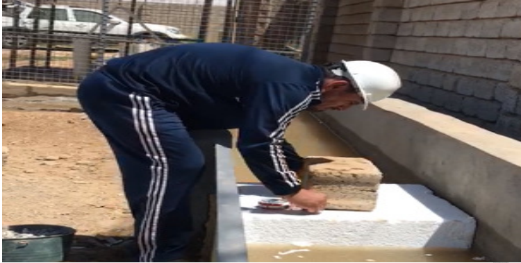
Fig. 5. Weight on the Floating Bridge test
