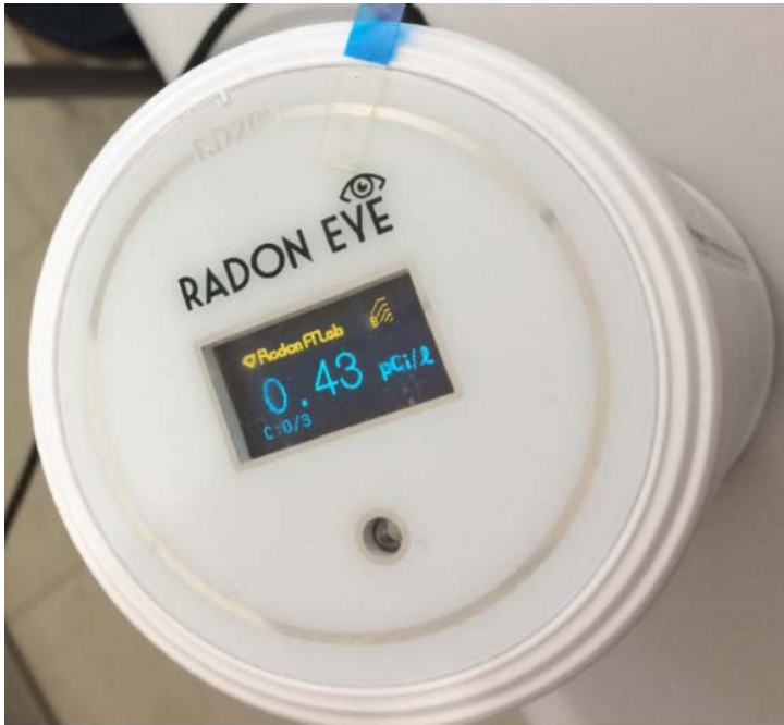
Fig 3 – Top view of Radon Eye RD200 ionization chamber used for monitoring radon gas [8]
