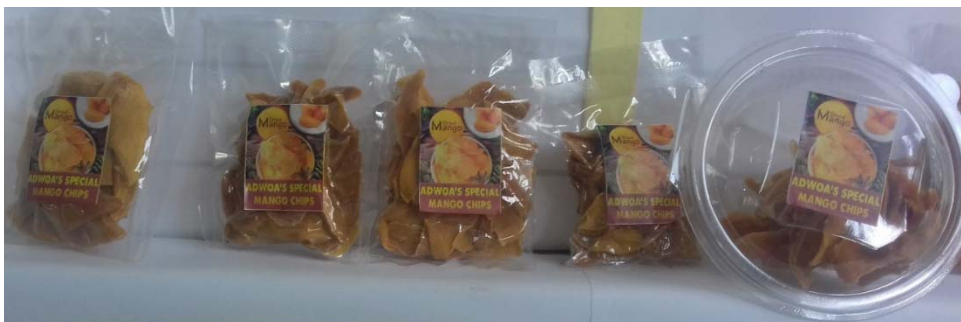
78 79 Figure 3: Differently processed, packaged and labeled mango chips stored at ambient conditions (L-R: sealed 80 polyethylene (0.085mm thick) (PolyEthyseal), vacuumed polyethylene (0.085mm thick) (PolyEthyvac), sealed 81 polypropylene (0.055mm thick) (PolyPropseal), vacuumed polypropylene (0.055mm thick) (PolyPropvac) and 82 plastic (clamshell) pack (PLASTICPACK)).
