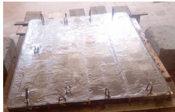
c-Casting of R.C. slab
