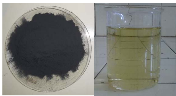
Figure 2: Electrode material powder and leaching filtrate
