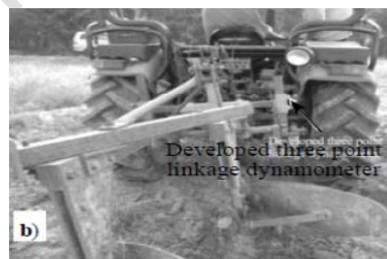
195 Fig. 5. a) Developed Three point linkage dynamometer, b) Field testing of the developed three point 196 hitch dynamometer with an implement (Tewari et al., 2012).
