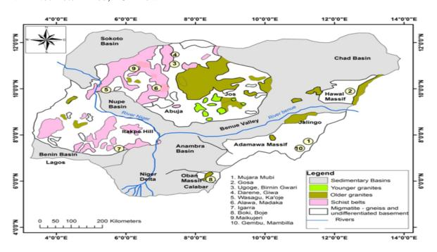
Figure 2. Simplified geological map of Nigeria Basement Complex showing the schist belts where manganese occurs (Modified after Woake *et al.*, 1987 and Danbatta, 2008).
