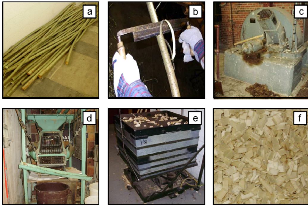
Fig. 2. Willow processing a) willow stems, b) debarking, c) chipping, d) pre-screen, e) final screening f) willow chips [31]
