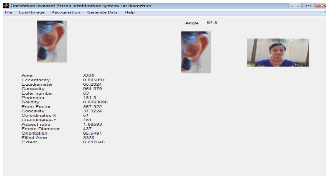
Figure 15. Person identification when head tilt at 67.5^{\circ}
