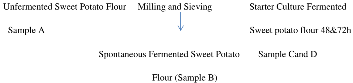
Fig 1: Flow diagram for the production of unfermented, spontaneous fermented sweet potato flour samples (Oluwole et al. , 2012) and starter culture fermented sweet potato flour.
