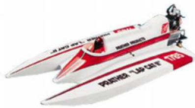
Figure 2.8: Tunnel hull RC boat (33)
