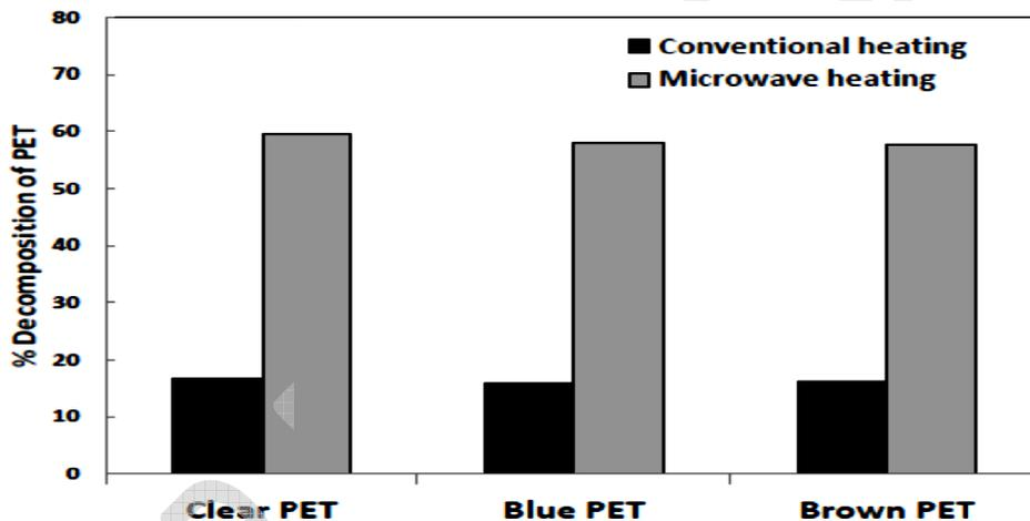
Figure 4: Comparison between conventional and microwave-assisted heating of PET decomposition in a propan-1-ol media.
