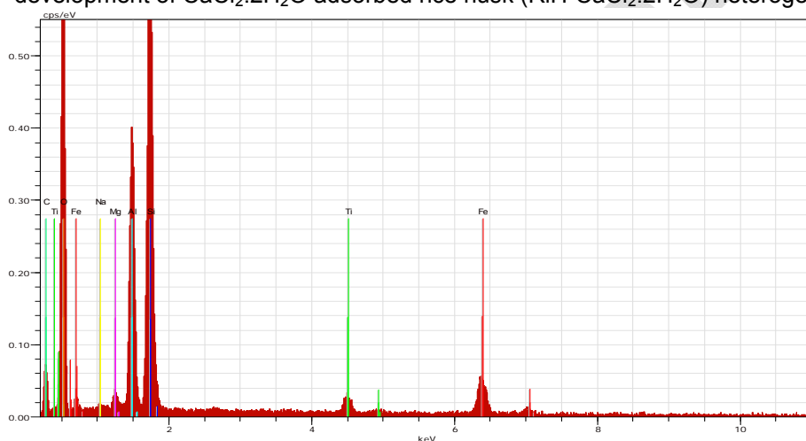
Figure 4. EDS Spectrum of rice husk (RiH)
