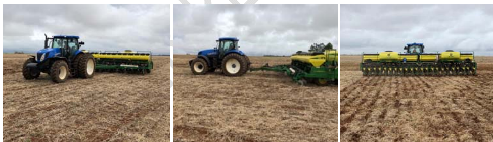
Figure 1. Frontal, lateral and posterior views of the tractor-sowing system, used in sowing of corn
