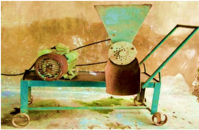
Plate 1: The machine showing pelletizing operation
