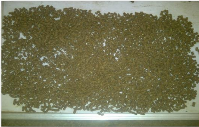
Plate 4: Pelletized fish feed of 6mm diameter.
