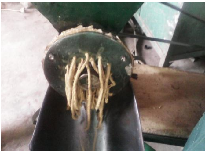
Plate 1: The machine showing pelletizing operation
