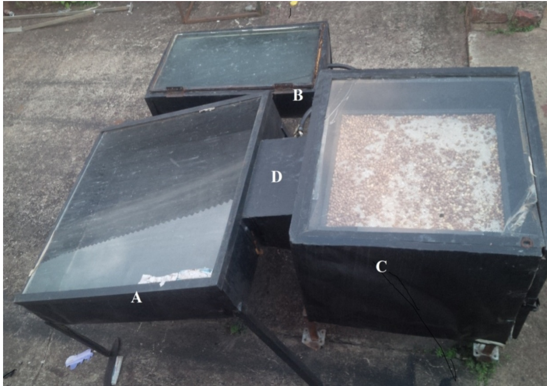
Fig 1: The Experimental Solar Dryer
