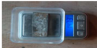
Fig. 3. Ultra-sensitive weighing balance used for weighing the carbon steel coupon
